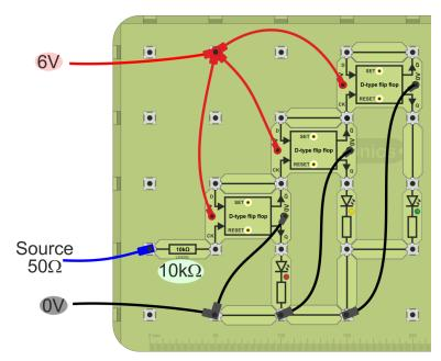
Each D-type flip-flop generates the pulse that triggers the next. Hence they change in sequence.
